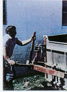
6: Two pins release the trailer assembly, causing it to swivel up and the tank to drop. Reinsert pins in upper slots to hold up the trailer.
